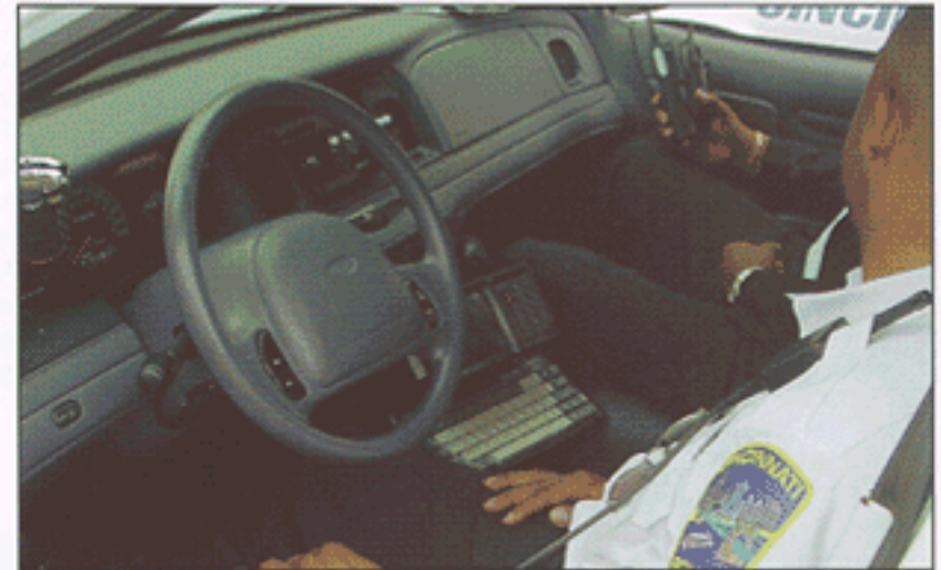
The Police Information Services Levy supports technology such as Mobile Data Terminals mounted in police cruisers, which provide access to information in local, state and national databases regarding wanted and missing persons, persons with protection orders, stolen vehicles and property, driver's licenses and criminal history.
